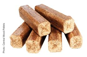
Over the last decade, the Brazilian forest industry began to produce wood pellets and briquettes, both for companies' internal use and to sell on the national and international markets. Pellets consist of sawdust that is compacted at high pressure and temperature, while briquettes are made by compacting sawdust, wood chips, and other forest biomass.
