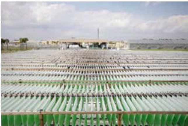
Algenol's photoreactor bags converting algae to ethanol at its Florida facility. Photo courtesy of Algenol.
