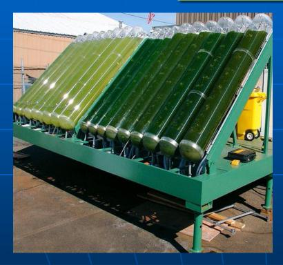
A Photo-Bioreactor in Translucent Tube from GreenFuels
