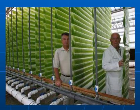
Global Green Solutions/Vertigro Vertical Photo Bioreactor System
